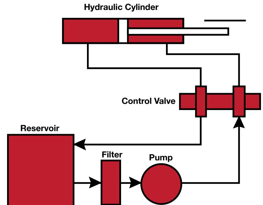
**Although systems are extremely power-dense, hydraulic actuators have the lowest energy conversion efficiency of the three actuator types. (Source: Exlar)**
