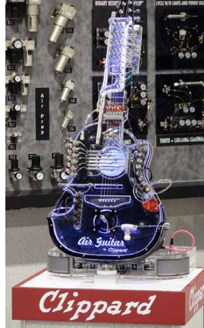
Clippard’s air guitar uses a combination of 5/16-inch and 5/32-inch air cylinders to strum its six strings. A half-inch-diameter cylinder provides percussion.
