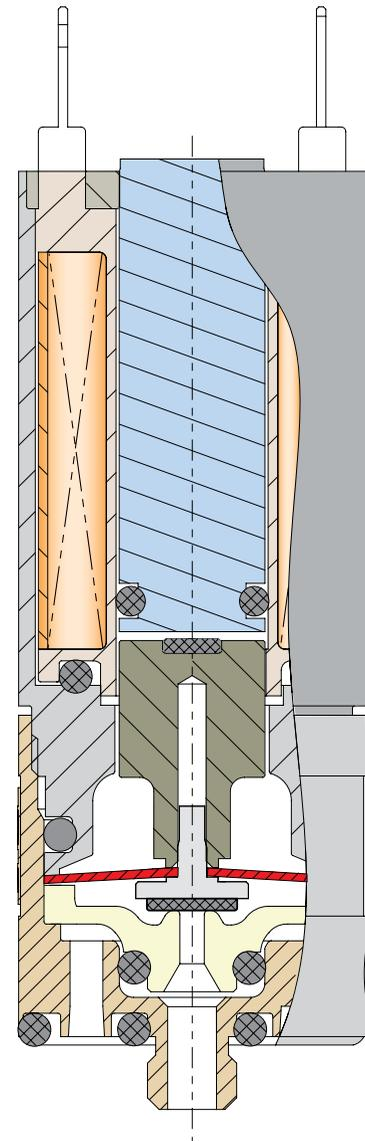
us to see what kind of magnetic pull we could generate.” Dave goes on to say that many coils were made in the attempt to optimize one. This led to an optimized solenoid needed for the valve. The process for determining the correct coil was enhanced by a coil calculator. The calculator, which was designed by Clippard’s engineering department, greatly reduced the design time and provided the exact specifications of the coil.
