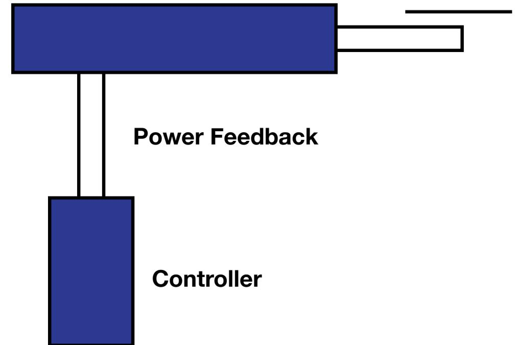
**Electromechanical systems offer a simplified mechanical solution, and fewer or no components are needed between the power source and the actuation component, which can create much higher energy efficiency.**
